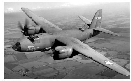
now designated AT-23s, had their armor and armaments, including their dorsal turrets, removed. A windlass was added to which the target sleeve itself could be attached and trailed behind the towing airplane.
