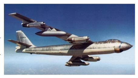
releasing its bomb load, adding to the bomb's flight time and giving the aircraft extra time to escape the blast effects of the bomb, particularly important if the bomb is a nuclear device. The problem with loft bombing was that its repetition in training stressed the airframe and could cause metal fatigue.
