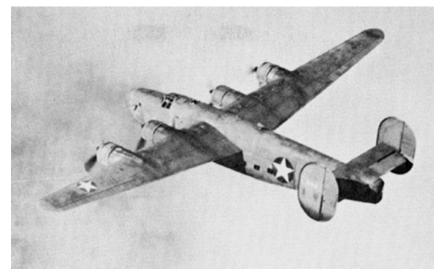
concluded that the airplane took off with its flaps extended, increasing its drag and making it impossible to quickly climb. In addition, the investigators determined that the landing gear and the flaps could not both be retracted at the same time, so the extended gear added to the already increased drag further increasing the difficulty of remaining aloft. It was Stone's thirteenth mission.
