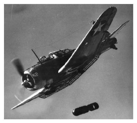
delivered their bombs on target not by relying on a highly technical, highly classified bombsight, but by simply aiming their aircraft directly at the target. As the bomber dove toward its target, the pilot could adjust his aim by tweaking the angle of his dive. This, of course, required practice.
