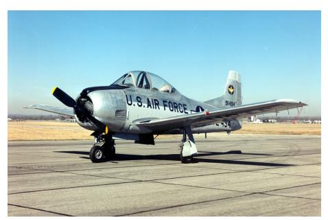
The T-28 was a twoseat, radial-engine trainer used by both the Air Force and the Navy. It was powered by a 1,425horsepower engine that could propel the aircraft to a maximum speed of 340 miles per hour. The Trojan would help prepare student pilots to transition to the even faster jets then in the Air Force inventory.
